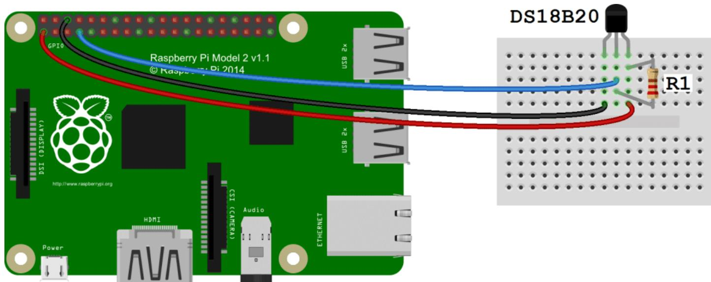
R1 is 4.7k ohm resistance for pulling up the voltage level
